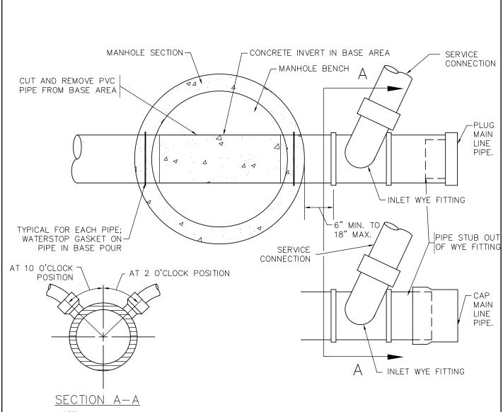
NOTE: TAPS IN STAGGERED CONFIGURATION AT 10 O'CLOCK OR 2 O'CLOCK POSITION.
