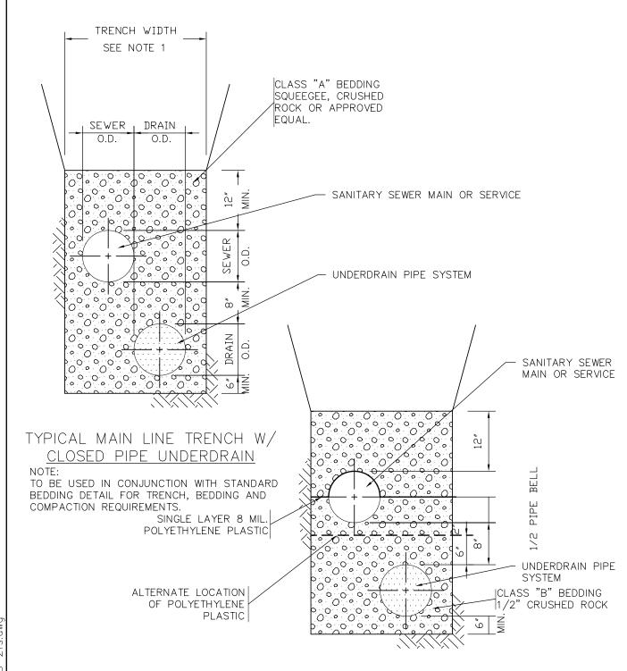
ALTERNATIVE MAIN LINE TRENCH W/CLOSED OR OPEN PIPE UNDERDRAIN
